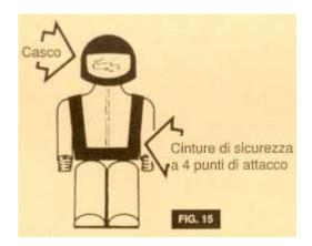
Obviously the anchor points on the aircraft structure must have been chosen to be robust and resistant. Use of this type of harness has particular importance in certain critical flight conditions such as:
